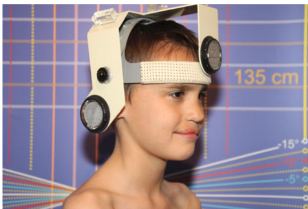
Fig. 1 The Keno®-cervical measurement instrument was used to measure cardinal plane active cervical range of motion during flexion, extension, lateral bending, and rotation
